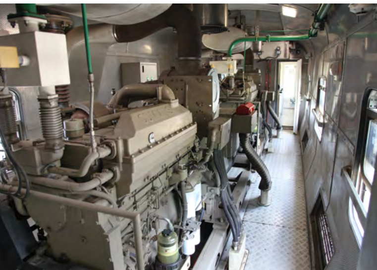
'Power cars' with dual 400 kW Cummins K19 generator sets are used to power the air conditioning on first-class trains.
