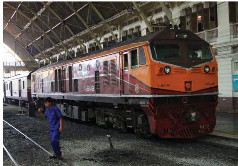
Cummins KTA50 is popular in the SRT fleet powering these General Electric locomotives.
