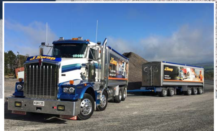
Top: A typical combination in NZ – 8x4 truck coupled to a five-axle trailer. Right: One of the 65 Kenworths that spearhead the Swap transport task.
