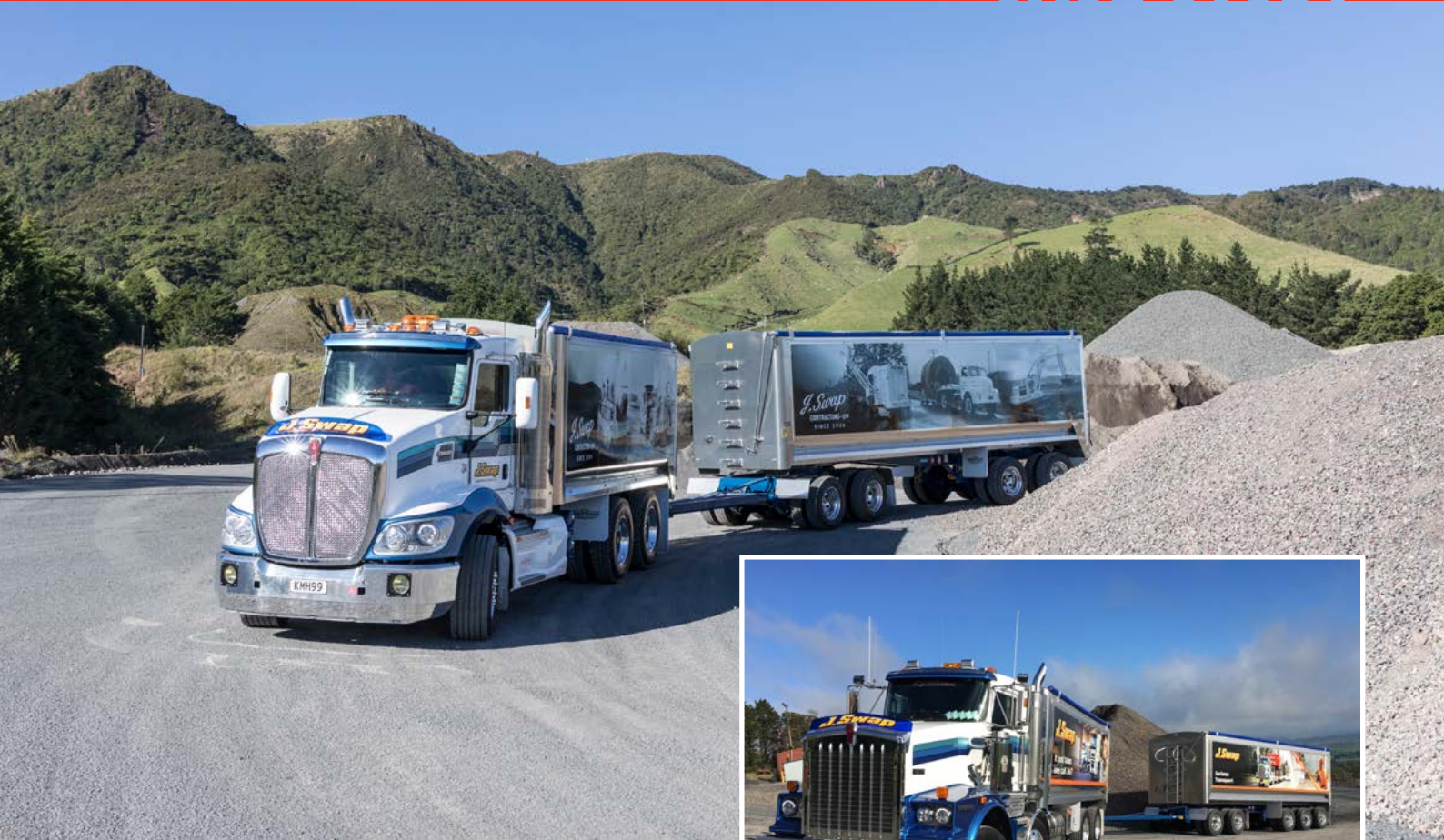
Top: A typical combination in NZ – 8x4 truck coupled to a five-axle trailer. Right: One of the 65 Kenworths that spearhead the Swap transport task.
